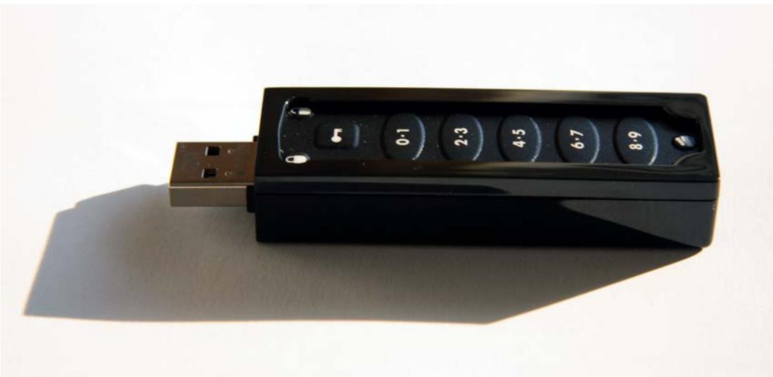
Fig. 2 Not ultimate as well: USB tokens and code-protected USB sticks (code protection, not data encryption)
