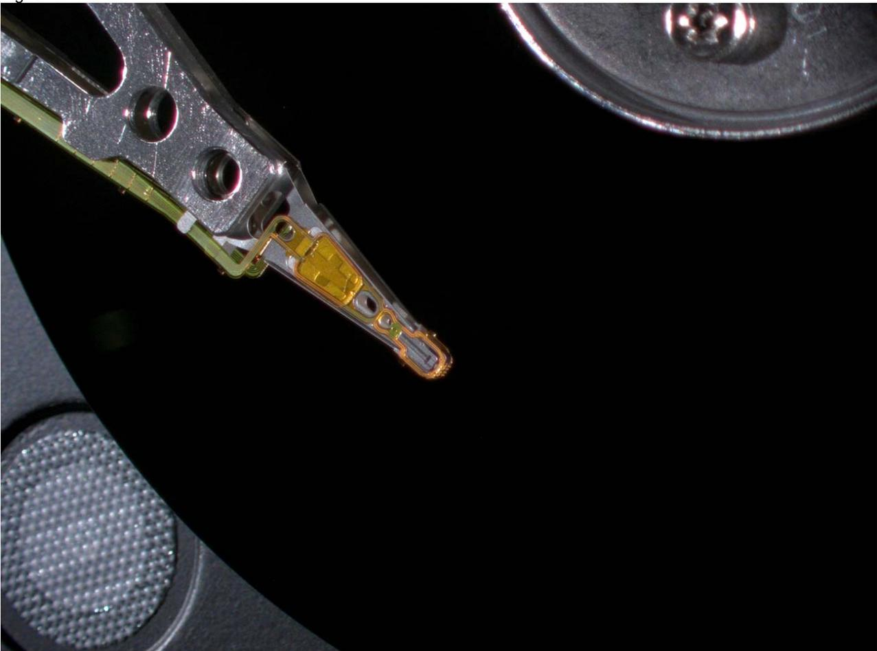
Fig. 6 Closeup on magnetic harddisk head
