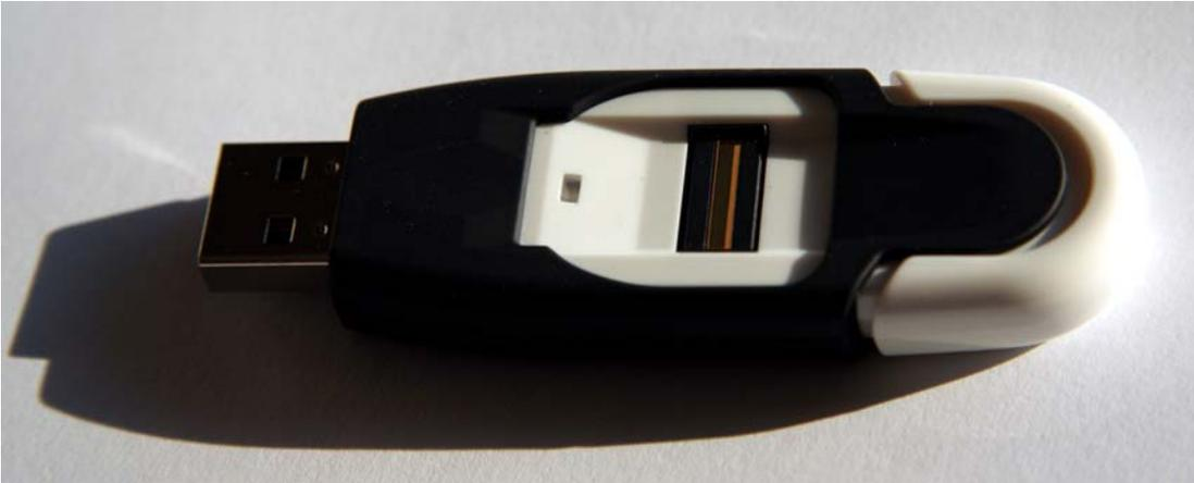
Fig. 1 Ultimate security is not possible to guarantee with fingerprint sensors (high False Acceptance Rate)
